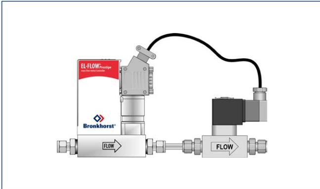
The digital output of the programmable pin 5 (9-pin sub-D connector) can be used to activate a shut-off valve. For instance, a shut-off valve can be programmed to close when the MFC's setpoint is zero, to ensure that the gas line is absolutely closed. Alternatively the valve may be activated upon a certain alarm value or when a preset counter value has been reached. This functionality makes the use of valve terminals superfluous.
