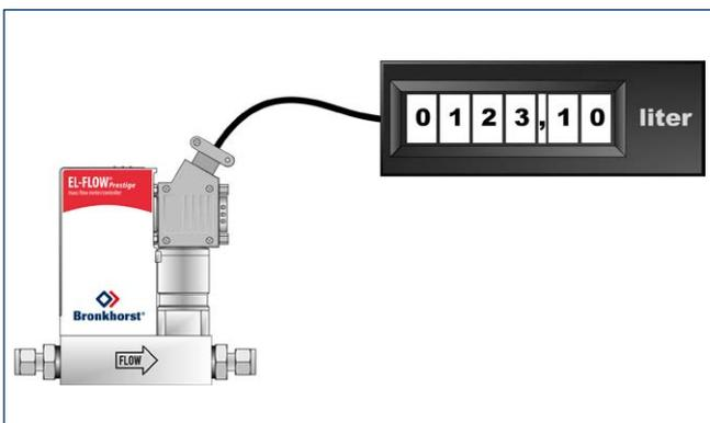
The programmable pin 5 (9-pin sub-D connector) can be set for a pulse output per quantity, as defined by the user. This pulse can be fed directly to remote totalizing counters, digital readout devices or control instrumentation.
