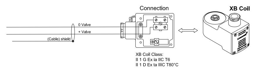
(Cable) shield <u>must not</u> be connected to the coil(housing)
