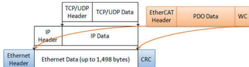
Data is communicated between master and slaves in the form of process data objects (PDOs). Each PDO has an address to one particular slave or multiple slaves, and this “data and address” combination (plus the working counter for validation) makes up an EtherCAT telegram. One Ethernet frame can contain multiple telegrams, and multiple frames may be necessary to hold all the telegrams needed for one control cycle.
