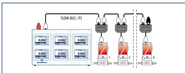
Alternatively only one display can be used to readout these instrument sequentially; model key for this option is E-8101-R-10-00-00
